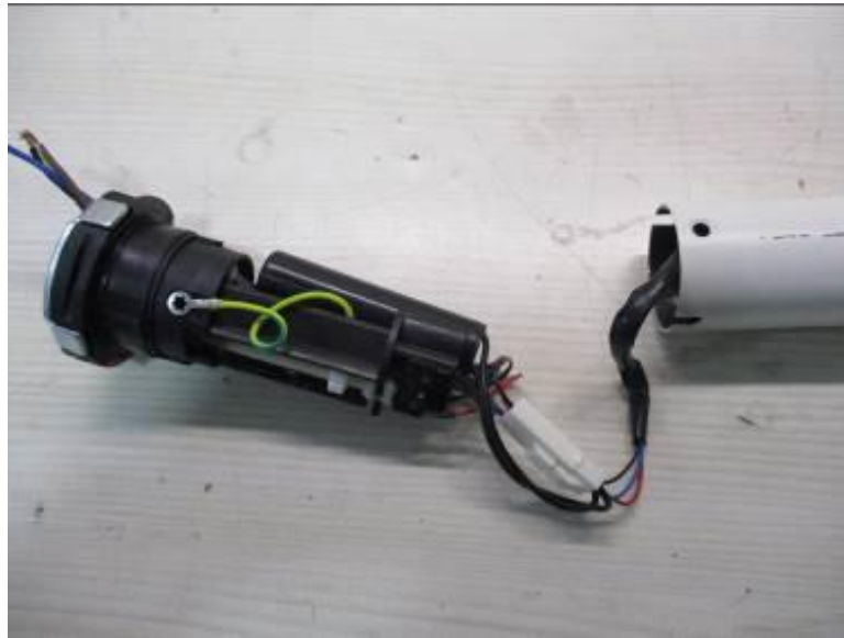
Photo 13. Shutter motor internal structure (up-down move button)
